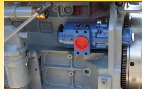
T20 installed on Deutz 1013 engine.
