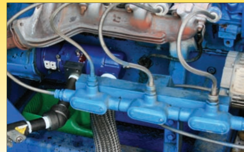
T20 installed on 5.9 Cummins engine.
