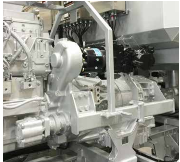
Logan SAE 600 series Direct Drive PTO's Mounted to a live PTO wing drive, sandwiched between a CAT 3412 Engine and an Allison 8900 Series Transmission. Logan PTO's are used to disconnect single and tandem pumps on an oil and gas vehicles.
