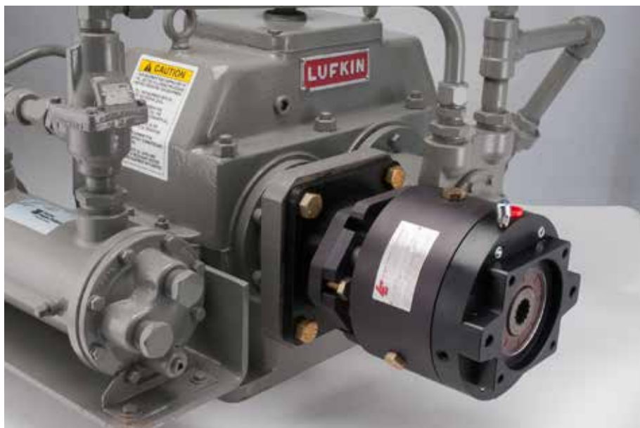
Lufkin Gearbox with Logan 600 Series Direct Drive PTO (600 lb. ft. / 1335 Nm) @ 200 psi. / 13.6 bar. The Logan PTO is positioned between a pump and gearbox, enabling power on demand for cold starts, and connect-disconnect applications.
