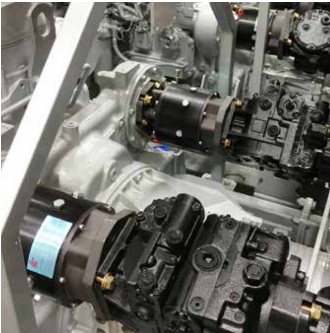
Close up of (4) Logan 600 series PTO's used to connect and disconnect the single and tandem pumps between jobs, or during on-highway trips to prevent pumps from overspeeding.
