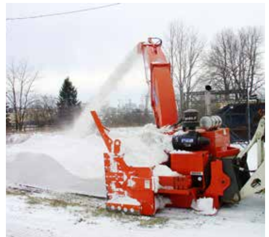
Wheel Loader Retrofitted with a Self-Adjusting™ Logan Bell PTO, originally used a mechanical, lever activated over center PTO
