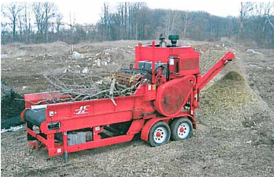
Shredder driven by 170 hp John Deere 6068T with Logan LC-211 transmits 963 lb. ft. (1305 Nm) @ 200 psi (13,8 bar)
