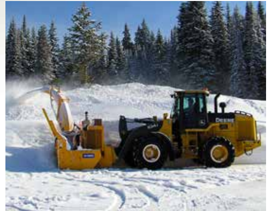
Wheel Loader equipped with a Logan Bell PTO clears a parking lot
