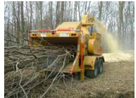
Feed / discharge system has 20" (50.8 cm) chipping capacity
