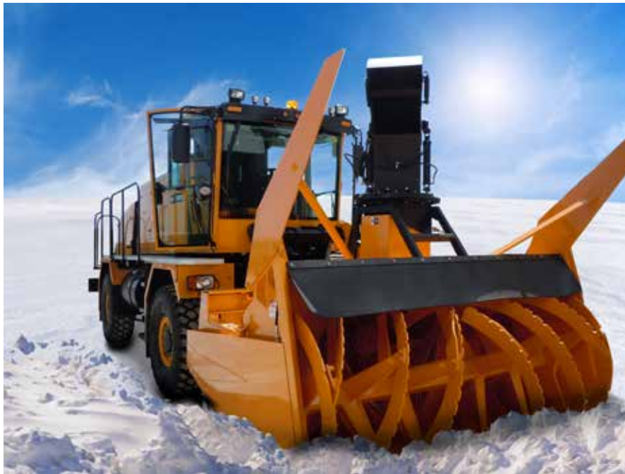
This Airport 700 HP Snow Blower is equipped with a Logan LC-318 Bell Housing PTO and is capable of clearing a 120" wide path of snow, moving 6000 tons of snow per hour
