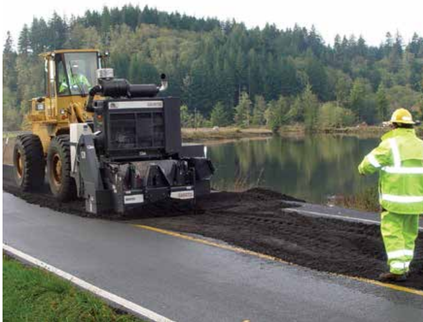
Milling machine equipped with 200 hp engine and LC211 PTO shown mounted on a wheel loader
