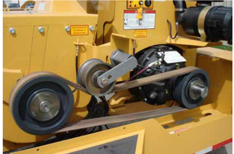
Logan PTO Clutch mounts directly to engine's SAE flywheel
