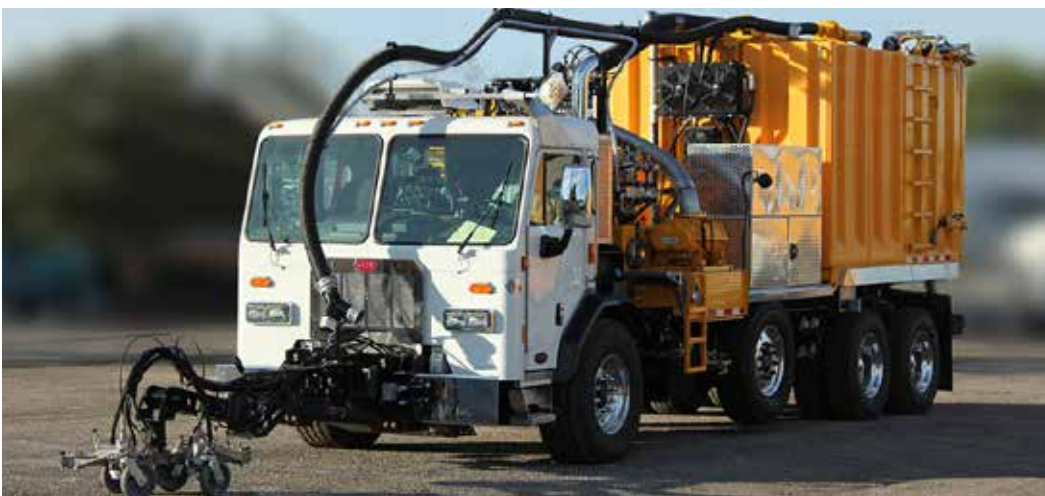
Waterblasting truck equipped with 375 HP Diesel Engine and an air / fluid actuated Logan LC-314 Bell Housing PTO for smooth engagement.
