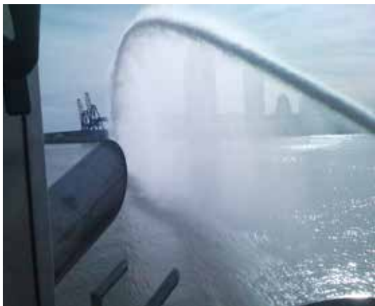
The pump system is capable of transmitting a 4" / 10cm diameter stream of water as far as 400 ft / 122 meters
