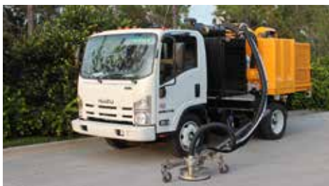
Medium Duty surface preparation truck equipped with Logan LC-211 Bell Housing PTO powered by a 200 HP Diesel engine.
