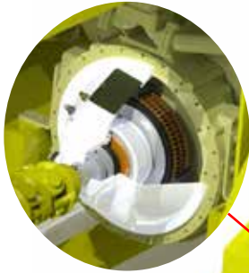
Logan LC-311 Bell Housing PTO 1446 lb. ft. (1960 Nm)
