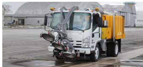
Heavy duty airport marking removal truck equipped with a Logan LC-311 Bell Housing PTO, with SAE No. 3 flywheel mount, powered by a 240 HP diesel engine.
