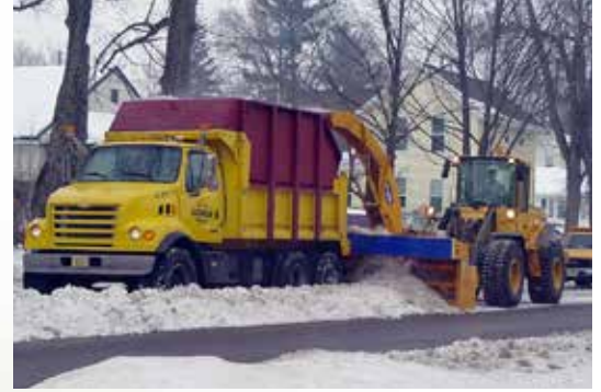
Municipal Loader using a Logan LC-314 Bell Housing PTO, which transmits 2702 lb. ft. (3664 Nm) of torque
