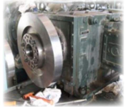
Clamp Hub on brake disc
