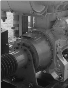
Wichita PTO mounted on Caterpillar diesel engine.
