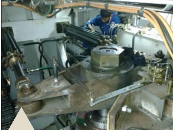
A 9-ton meter steering arrangement for a twin screw tug with electronically synchronized rudder (no mechanical tie bar to the second rudder).
