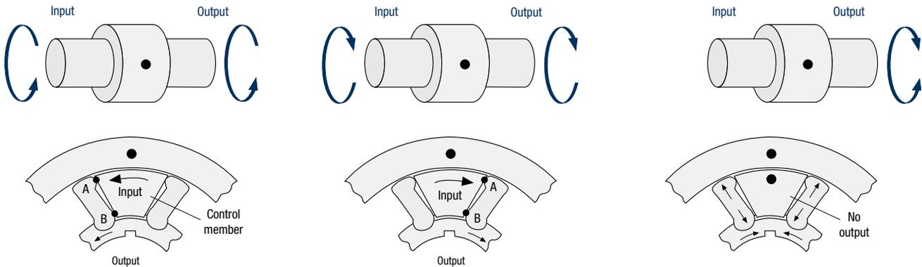
The control member projects between each pair of opposing sprags and when driving torque is applied to it, each projection first contacts a sprag at point "A" to disengage the sprag from the **outer race**. Then, the **control member** drives against the sprag at point "B" to transmit driving torque directly to the **output member**.
