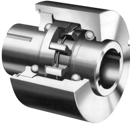
Available in six sizes, the Formsprag RL Clutch is a sprag type no-back which permits transmission of driving torque from input to output shaft in both directions of rotation, but restrains any feedback torque of the driven load from rotating the output shaft in either direction.
