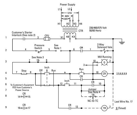
Normal mill starting procedure is to bring the motor up to operating speed and then engage the clutch to accelerate the mill. Airflex offers a simple, but very reliable system for clutch control. The system consists of two parts: the pneumatic and electrical portions.
