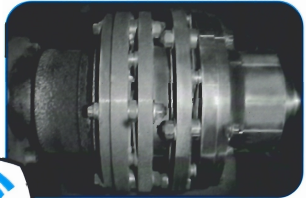
UltraFLEXX size 250 running a 100 HP pump at 3,600 RPM
