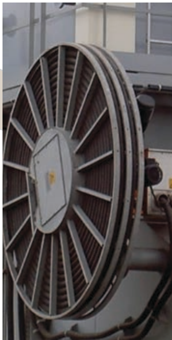
Double Monospiral Spool , with two identical cables with large cross-sections.
