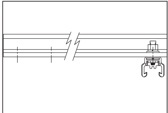
Figure 13-2 Flange Support Brackets
